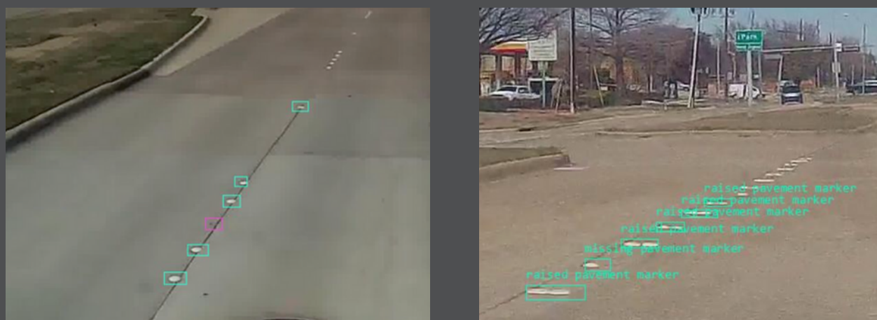
Figure 13. This figure shows two different examples of missing raised pavement markings
